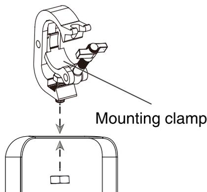
To clamp the fixture to a truss:
